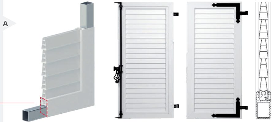
Lames horizontales, standard, blanches. Renforts aluminium en standard.
